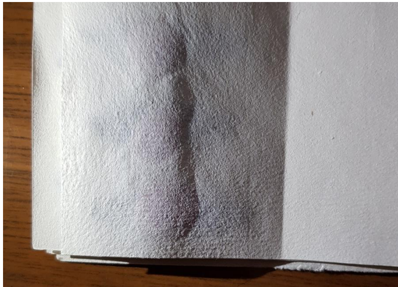
Figure 53: Deformation around the samples of the reconstruction. Very similar to the deformation in the Lakenhal sample books. Photograph taken by Margot Terpstra.
