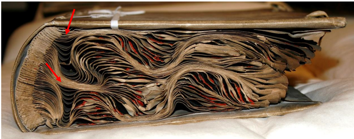
Figure 44: Bottom edge of Lakenhal sample book 1312.9. Red arrows indicating how a small fold or bump in the paper will increase in severity. Photograph taken by Margot Terpstra.
