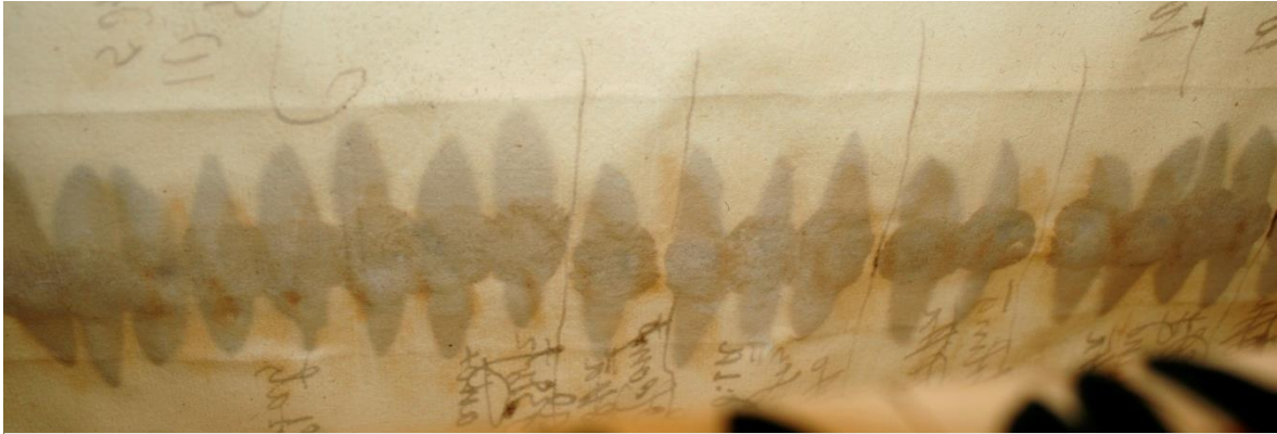
Figure 49: Verso of a page from Lakenhal sample book 1312.3. In comparison to the verso side of other sample books, these samples shine through the paper. The sealing wax appears to have left a tideline. Photograph taken by Margot Terpstra.
