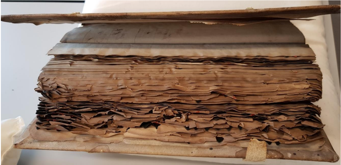
Figure 14: Fore-edge of Lakenhal sample book 1312.9 showing surface dirt, brittleness of the paper and edge tears. Note how the pages that lie deeper into the bookblock have less abrasion and surface dirt. Photograph taken by Margot Terpstra.
