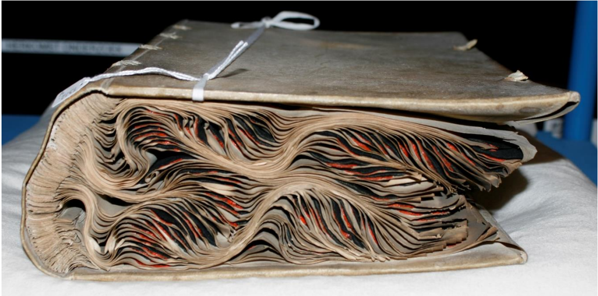
Figure 2: Bottom edge of Lakenhal sample book 1312.4. Relatively mild case of the ‘wave’-pattern deformation. Photograph taken by Margot Terpstra.
