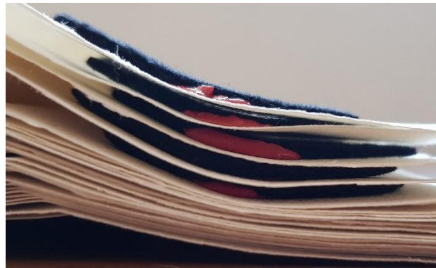
Figure 28: The samples and the paper take on a slight curve because they are pressed down using a finger. Photograph taken by Margot Terpstra.
