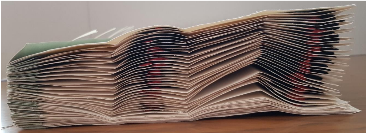
Figure 29: Closed reconstruction. The column on the fore-edge shows the first signs of deformation and tend to bend inwards towards the spine. Photograph taken by Margot Terpstra.
