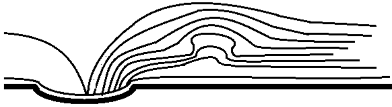
Figure 45: A small fold or snag in the paper gets exaggerated by the pages lying on top. Schematic made by Margot Terpstra.
