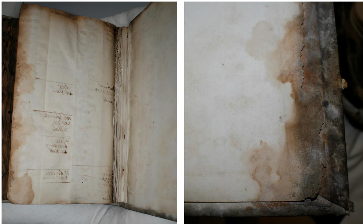
Figure 48: Signs of moisture in the paper of Lakenhal sample books 1312.8. Left: Tidelines on the last page of the sample book. Right: Tidelines on parchment and on past down against the back board, bottom corner. Photographs taken by Margot Terpstra.
