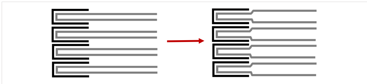
Figure 35: The guards create empty spaces between the pages where the paper is more free to move to than it would be in ‘solid’ bookblock. Note that the state on the right is not fixed, and the paper will keep moving. Schematic made by Margot Terpstra.
